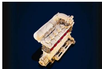
Le Mans race engine built by Aston Martin using 3D printing technology
